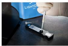
Dispense 100 μL sample/reagent mixture into the cartridge.
