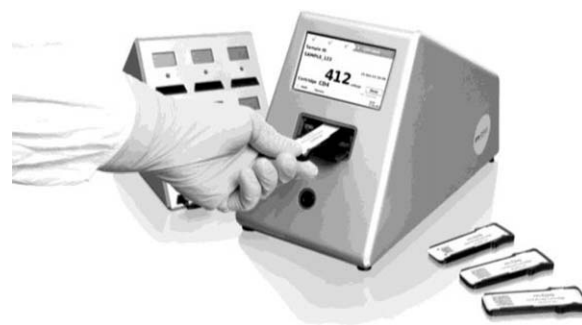
FIG. 3. MBio CD4 System showing cartridge being inserted into the Reader. The MBio Rack used for cartridge and timing management is shown in the back.
